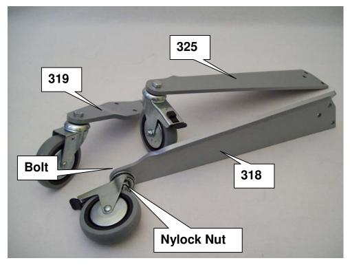
**Step 3**. Base Assembly, Parts required- 318, 319, 325 & 316 Secure all parts as shown using 8x20mm CHB's. The Joggle (kink) in Part 319 needs to be orientated upwards as shown.
