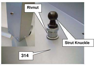
**Step 5.** Parts Required- 314 & 317. Slide 317 into 314 then screw the 8mm hand wheels into the Rivnuts through the slots on the side of 314.
